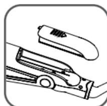
Before any filling, remove the tank [I] by sliding it in the direction indicated by the arrow, without lifting.
